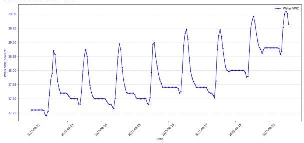
All moisture sensors provide volumetric water content (VWC) data represented in percentage format, as shown above. This data remains unstandardised and exhibits variations based on the specific sensor and the type of medium being measured. Consequently, growers face challenges in utilising this data to accurately assess whether the medium is experiencing over-irrigation or under-irrigation.
