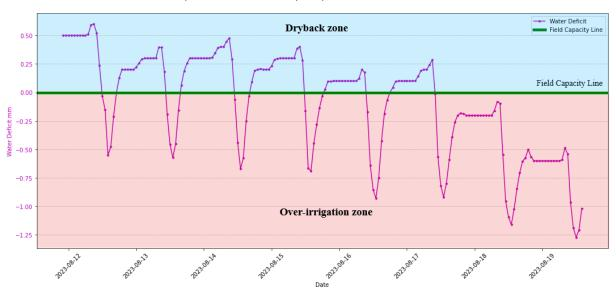
The deficit-surplus chart displayed above is derived from VWC moisture data. It is normalised using the field capacity or optimum water holding capacity of the medium, which is represented as a zero line and is color-coded in green. When the reading falls below the field capacity line, it indicates that
